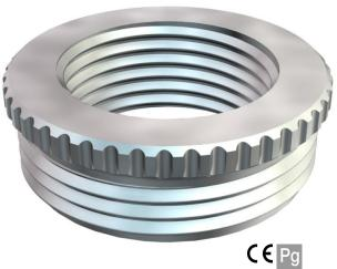
Reduction (Part H) to DIN 46320, with Pg thread to DIN 40430, as a transition from a PG thread hole to a smaller cable gland.  $^{\star}$  Prices according to DEL notation.
