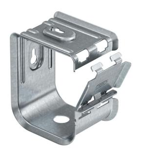
Metal grouped support for high mechanical stability, even in case of fire. Suitable for safe mounting above fire protection ceilings. Also approved as a cable-specific variant for the maintenance of electrical function to DIN 4102 Part 12. For wall and ceiling mounting. Lock can be opened without tools. Detailed information on the approved routing variants can be found in the appropriate testing documentation.
