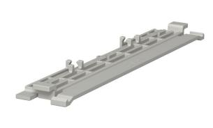
Cover clip for better and easier laying of lines in the WDK trunking. The cover fixing device can be moved along the entire length of the trunking. The cover clip is locked on one side and moved forward. This provides a 30° opening, meaning that cable routing is very simple.
