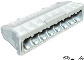
Screwless terminal to connect single-strand cables. Nominal cross-section: 8 x 0.5 mm<sup>2</sup> to 2.5 mm<sup>2</sup> single-wire conductor
