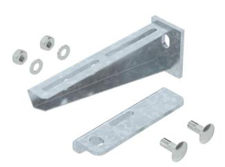
Bracket for mounting on suspended supports or as wall bracket for cable tray routing type above fire protection ceilings and for routing types with cable ladders and cable trays for the maintenance of electrical function according to DIN 4102 Part 12. The brackets are supplied ready-mounted.
