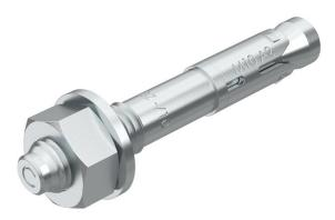
Bolt tie BZ with reduced anchoring depth for the anchoring of medium-duty to heavy-duty loads, both in cracked and non-cracked concrete. It combines high approved loads with small edge distances and axial spacings. European Technical Approval ETA-99/0010, including characteristic values under fire exposure to fire resistance R 120.
