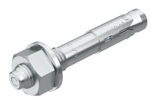
Bolt tie BZ with reduced anchoring depth for the anchoring of medium-duty to heavy-duty loads, both in cracked and non-cracked concrete. It combines high approved loads with small edge distances and axial spacings.
