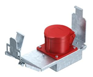
Device support of nominal size 3 with a CEE plug connection 16 A for installation in service outlets and cassettes of nominal sizes R7, 9 and R9. Device support with protective housing and strain relief. Required minimum installation depth: 190 mm when using a straight connector and 160 mm when an angled connector is used.
