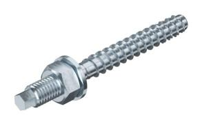
Bolt tie for direct mounting without additional anchors in cracked and uncracked concrete and masonry. With connection thread and washer to accept large loads. Suitable for fastening suspended loads from suspended supports and wall brackets in push-through mounting.
