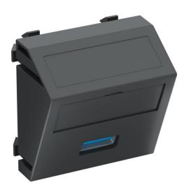
Multimedia support with one USB 3.0 connection socket, slanting cable outlet, with labelling panel, USB 3.0 type A socket with screw connection. Support plate with locking fastening, suitable for horizontal and vertical installation in the system environment.
