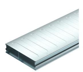
Underfloor duct (2 piece) for routing cables in screed-covered underfloor systems, according to EN 50085-2-2. Removable and continuously lockable trunking lid. With separating retainer in the trunking base. Only compatible with the UZD250-4/350-4.
